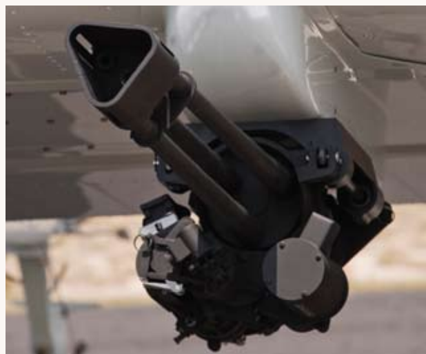
The AT-802U, equipped with the 12.7 mm GAU-19/A three-barrel Gatling gun. The LongSword is easily configurable to carry a wide variety of weapon systems.
