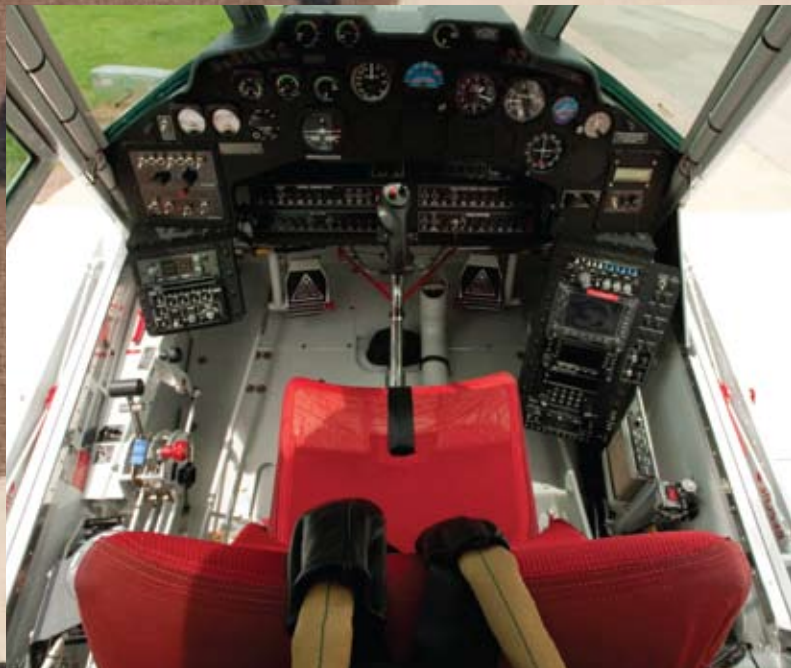
The AT-802U crew is protected by ballistic cockpit armor, crash-worthy seat and Am Safe inflatable restraints. The instrument panel is easily tailored to user needs and is NVG compatible.
